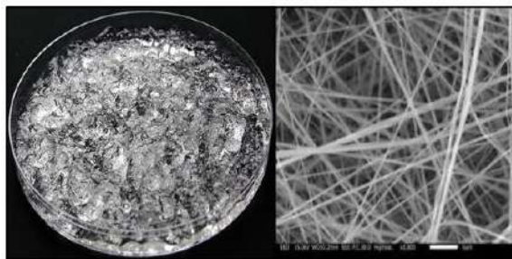
Figure 8. Cellulose nano fibers and TEM image of CNF
