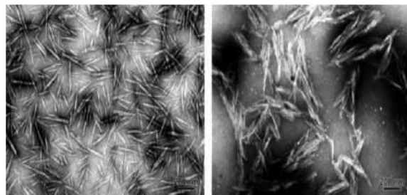
Figure 9. TEM images of Cellulose nano whiskers (CNW)
